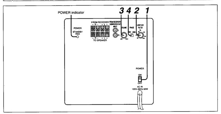
Set the low pass filter, volume and phase to suit characteristics of the front speaker and subwoofer combination.
